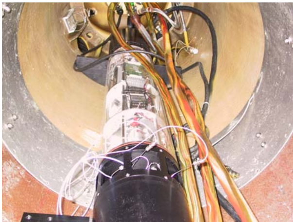
Figure 3. Mass spectrometer in ARCS vehicle.
