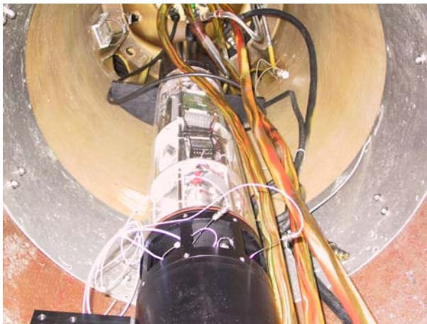
Figure 3. Mass spectrometer in ARCS vehicle.
